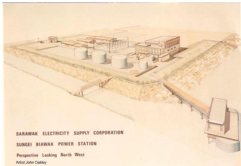
This was a diesel powered station with river water cooling. My Company designed the Mechanical, Electrical and Civil works. Construction was undertaken by specialist Contractors.
