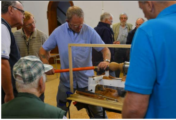
Deep hollowing on a small lathe at a practical evening
